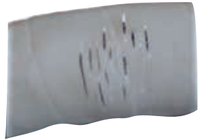
Hose with cover cracks due to age or the effects of ozone. Hose covers over time harden and should be replaced if this condition is found. (note: if boat has an ozone generator on board this could accelerate this condition
