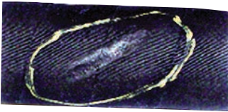
Hose cover melted due to contact with high heat of hot engine parts
