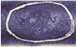
Hose with cover charred area from high heat or extreme aging due to heat or ozone
